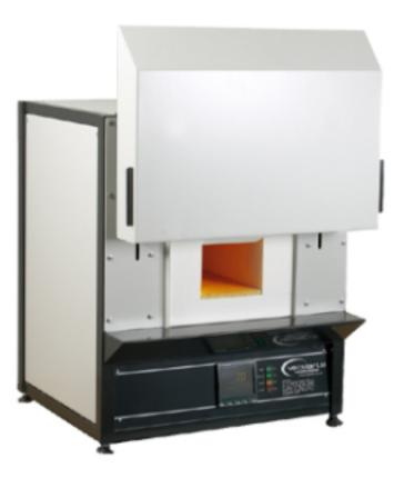
Our high temperature XF range of chamber furnaces are equipped with Molybdenum Disilicide elements positioned vertically down the sides of the chamber, this provides excellent temperature uniformity and rapid heat up times.
