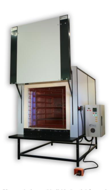
Vecstar design and build industrial fan assisted ovens designed and fabricated to specific customer requirements. Heat is provided via high quality mineral insulated, metal sheathed elements. All our fan assisted ovens come with a stainless steel chamber. Natural convection ovens are also available at customer request. Our ovens are available with a continuous operating temperature of up to 750°C (1380°F). We are able to provide 9 point UKAS accreditation to AMS 2750D at customer request.
