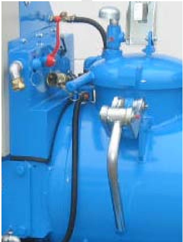
Air armature with upper and lower air controls. Lid with safety valves
