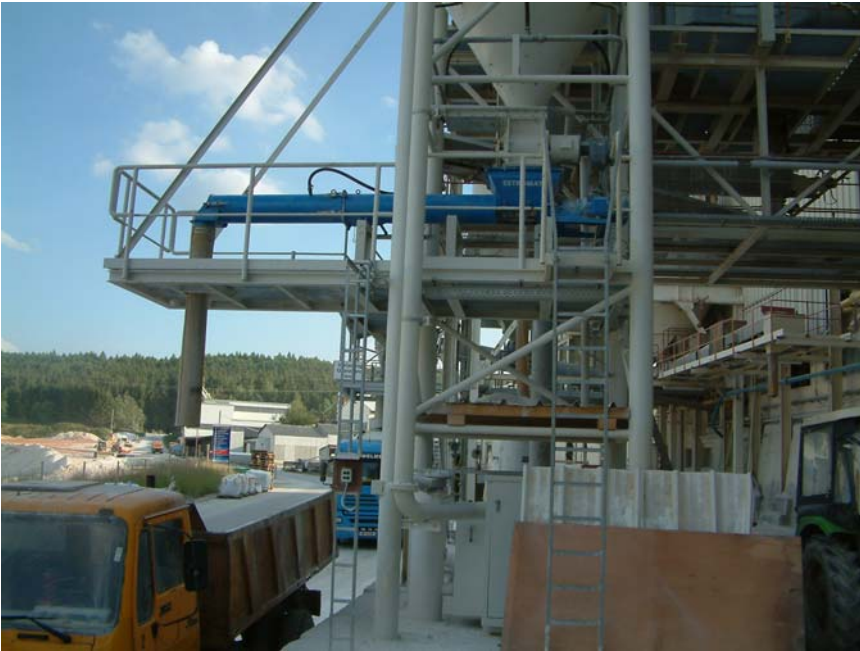
ESTROMAT 403 application for mixing powder residuals from sand classification unit
