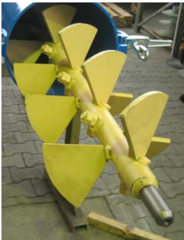
ESTROMAT 403 application for mixing powder residuals from sand classification unit
