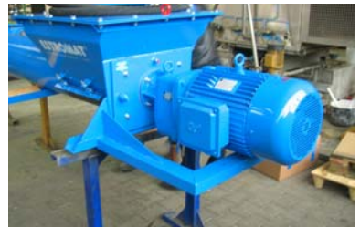
Different gear motors with a power of 7,5 up to 45kW can be delivered for special applications according to the material to be mixed.
