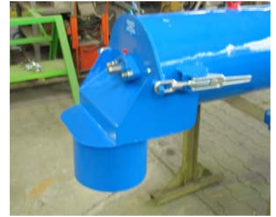
View to mixer material outlet with tube reduction
