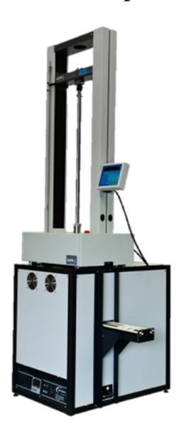
Our Hot Mor Furnaces are designed and manufactured to customer specifications. Model shown has a lloyd material testing unit. The furnaces are designed with a maximum temperature upto 1700°C. For more information please contact us. <u>Click here</u> for contact details.
